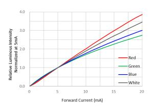
Fig.4 Relative Luminous Intensity vs. Forward Current
