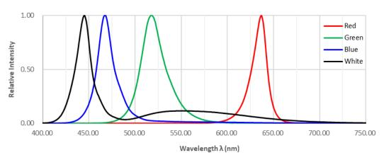
Fig.1 Relative Intensity vs. Wavelength
