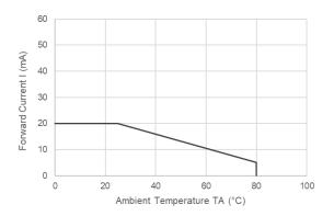
Fig.3 Forward Current Derating Curve
