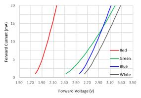
Fig.2 Forward Current vs. Forward Voltage
