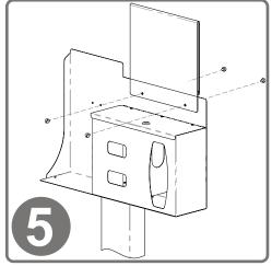
To mount the MP-075 Sign Holder, align the mounting holes of the holder with the holes on the top front of the dispenser. Attach using (2x) barrel screws included with sign holder.
