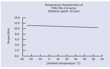
rated torque in this document) varies according to the ambient temperature. As the temperature increases, the torque decreases, and as the temperature decreases, the torque increases. This is because the viscosity of the silicone oil inside the damper varies according to the temperature. The graph to the left illustrates the temperature characteristics.
