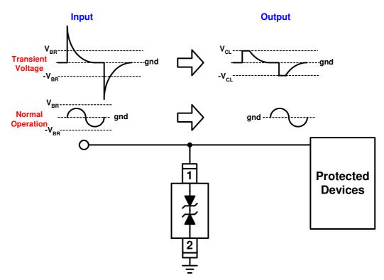
Fig. 1 ESD protection scheme by using AZ5925-01H.
