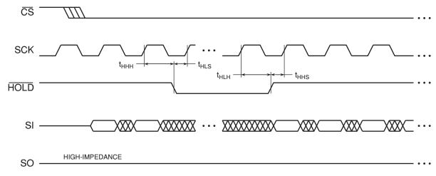
**Figure 14-5.** HOLD Timing – Serial Output
