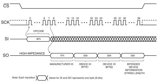
Figure 12-1. Read Manufacturer and Device ID
