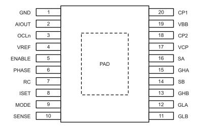
Package ES, 20-Pin QFN Pinouts
