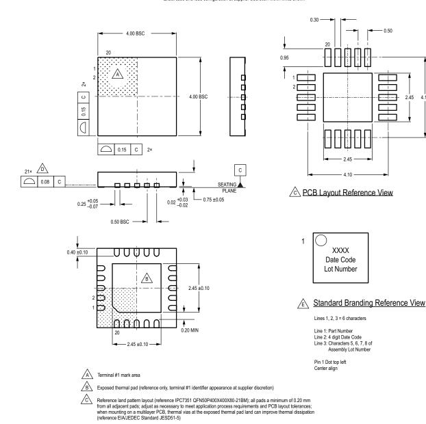
D Coplanarity includes exposed thermal pad and terminals Branding scale and appearance at supplier discretion.
