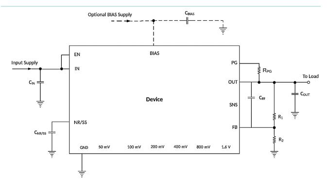
Figure 10 Adjustable Operation
