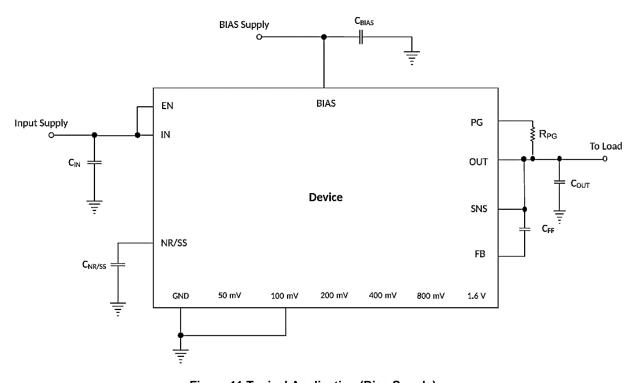
Figure 11 Typical Application (Bias Supply)
