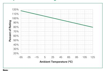
Rerating depicted in this curve is in addition to the standard derating of 25% for continuous operation.
