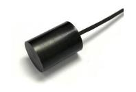
A240B works as a signal transmitting and receiving unit. This ultrasonic transducer is suitable for gas flow detection with high sensitivity, low noise, low ZFD (zero flow drift), high precision as well as exceptional reliability. In particular, the transducer housed with PVDF material is FDA compliance and free from corrosion by chemical solvent.
