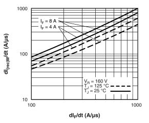
Fig. 8 - Typical dl<sub>(rec)M</sub>/dt vs. dl<sub>F</sub>/dt
