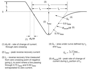
Fig. 10 - Reverse Recovery Waveform and Definitions
