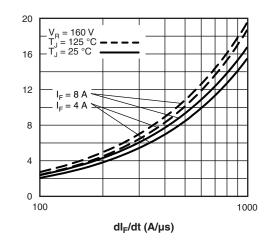
Fig. 6 - Typical Recovery Current vs. dl<sub>F</sub>/dt
