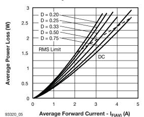
Fig. 5 - Forward Power Loss Characteristics
