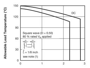
I<sub>F(AV)</sub> - Average Forward Current (A) 93279\_04 Fig. 4 - Maximum Allowable Lead Temperature vs. Average Forward Current
