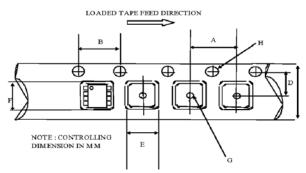
CARRIER TAPE DIMENSION FOR 16SOICW Metric Imperial Min Min Max Code Max 12.10 4.10 11.90 0.476 0.468
