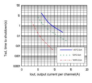
Figure 11 – Tsd (s) Vs I out (A) 2 channels on
