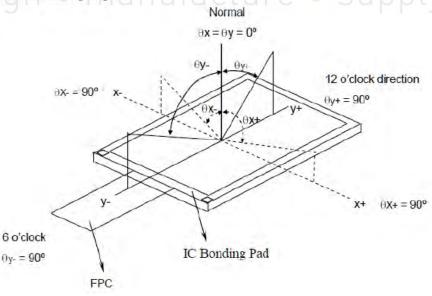
Note 8: Optical characteristic measurement setup.
