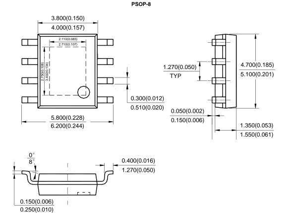
Note: Eject hole, oriented hole and mold mark is optional.
