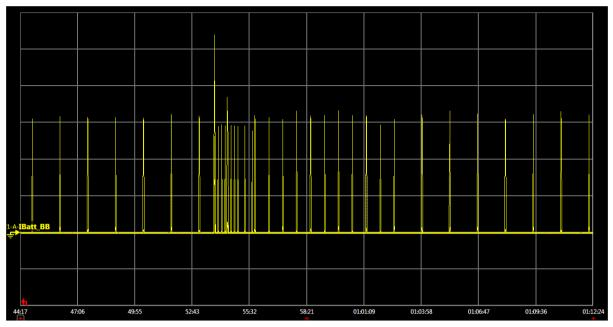
Figure 6. eDRX Power Consumption Profile Interruption
