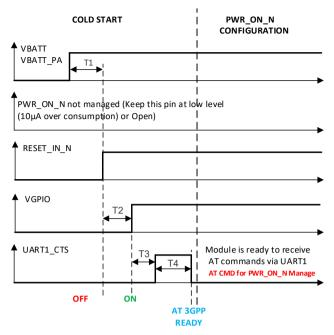
Figure 15. Power Up Sequence with PWR\_ON\_N Cold Start
