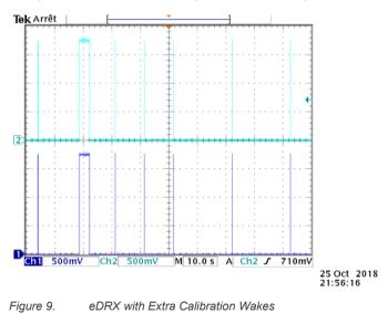
Eventually, a stable eDRX wake repeats every cycle without extra wakes. In the following figure, a PTW of 1.02 is used with a cycle of 81.92s.
