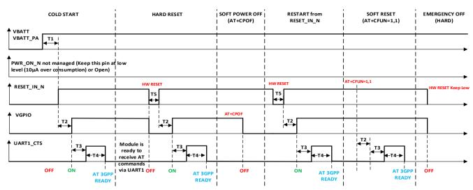
Figure 14. Power Up and Power Down Sequence without PWR\_ON\_N
