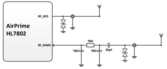
Figure 24. Antenna Connection
