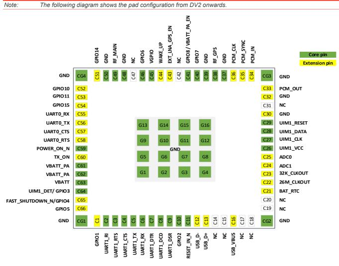
Figure 3. Pad Configuration (Top View through Module)
