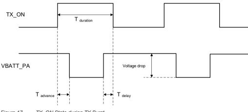
Figure 17. TX\_ON State during TX Burst
