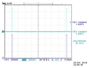
Figure 10. Stable eDRX Cycle of 81.92s after Calibration
