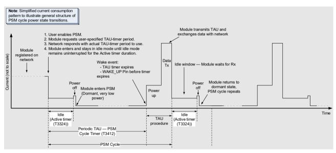
Figure 4. PSM Example (Simplified)
