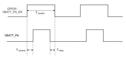
Figure 18. VBATT\_PA\_EN State during RX/TX Windows
