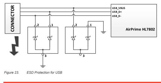
Note: It is not recommended to have an ESD diode with feedback path from USB\_VBUS to either USB\_D+ or USB\_D-.
