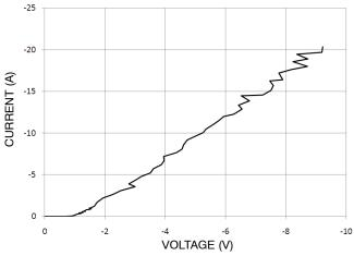
Figure 5. Negative TLP I-V Curve
