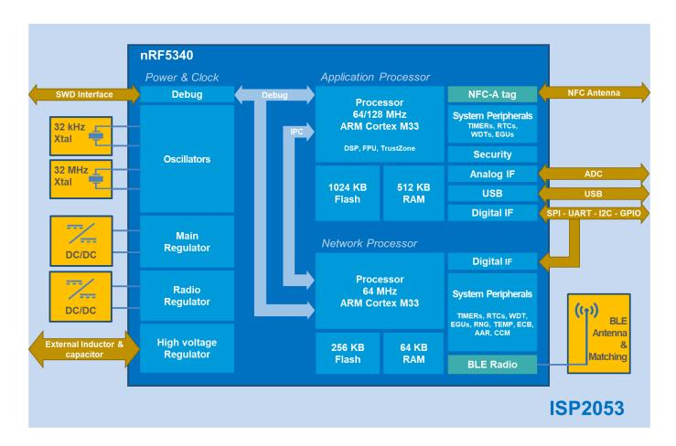
The application processor has 1 MB Flash, 512 KB RAM, a floating-point unit (FPU), an 8 KB 2-way associative cache and DSP instruction capabilities. The network processor is optimized for low power and offers 256 KB Flash and 64 KB RAM. In term of security, the Arm TrustZone provides trusted execution, the Arm CryptoCell-312 provides hardware-accelerated cryptography together with a root-of-trust and secure key storage management.
