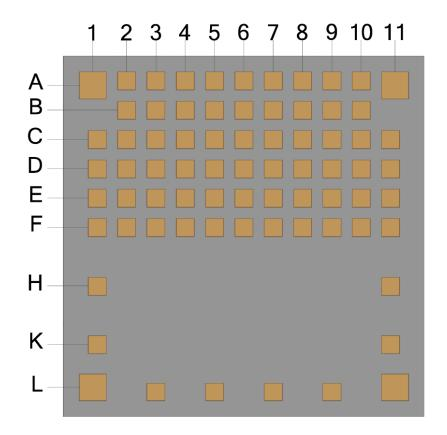
ISP2053 pad placement and pin assignment for the LGA QFN package
