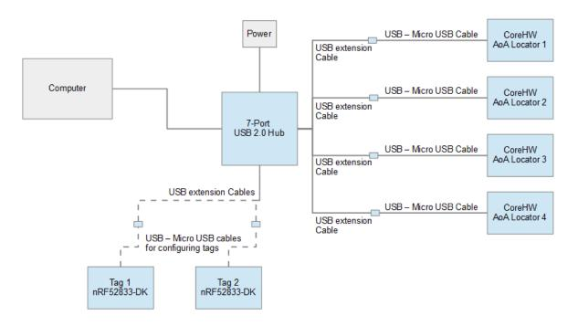
Gen1 locators can be installed e.g. on ceiling (mounting on floor, wall, 45 degrees from floor and 45 degrees from ceiling are also supported) of a room and connected via USB to Windows 10 PC running proprietary CoreHW AoA Demo software. PC Demo software can be used to demonstrate AoA Tag position estimation based on Angle-of-Arrival data.
