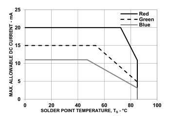
The preceding maximum forward current graphs based on ambient temperature  $(T_A)$  are with reference to the thermal resistance  $R_{\theta J-A}$  in the following table. See Precautionary Notes for more details.
