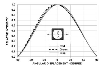
Figure 11: Radiation Pattern for Y-Axis
