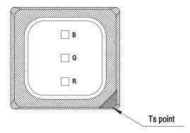
$T_S$  can be easily measured by mounting a thermocouple on the soldering joint as shown in preceding figure, while  $R_{\theta J\text{-}S}$  is provided in the data sheet. Verify the  $T_S$  of the LED in the final product to ensure that the LEDs are operating within all maximum ratings stated in the data sheet.
