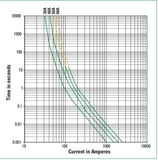
For 50A, 60A rating, it may not break current consistently when overload current is less than 200% ln  $\,$ (represented by dotted portion of this time-current curve), as maybe arc current continuously pass-through fuse under this condition. Do not recommend to use conditions of below 200%ln overload.
