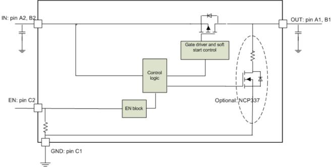
Figure 2. Block Diagram
