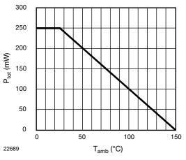
Fig. 3 - Admissible Power Dissipation vs. Ambient Temperature
