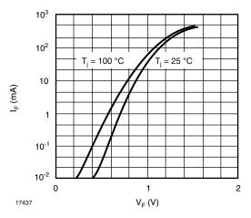
Fig. 1 - Forward Characteristics
