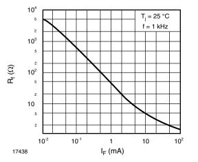
Fig. 2 - Dynamic Forward Resistance vs. Forward Current
