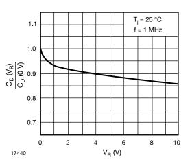
Fig. 4 - Relative Capacitance vs. Reverse Voltage
