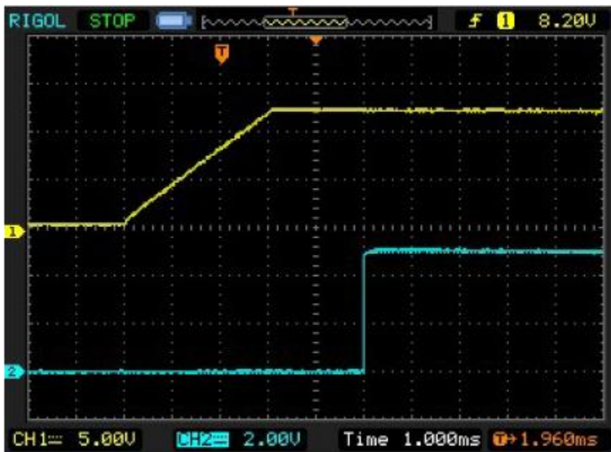
Figure 4. RESET goes high 2.4ms after V_{OUT} exceeds 11.4V.
