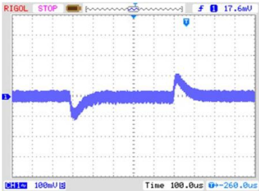
Figure 14. Load transient response when load steps between 600mA and 1A.
