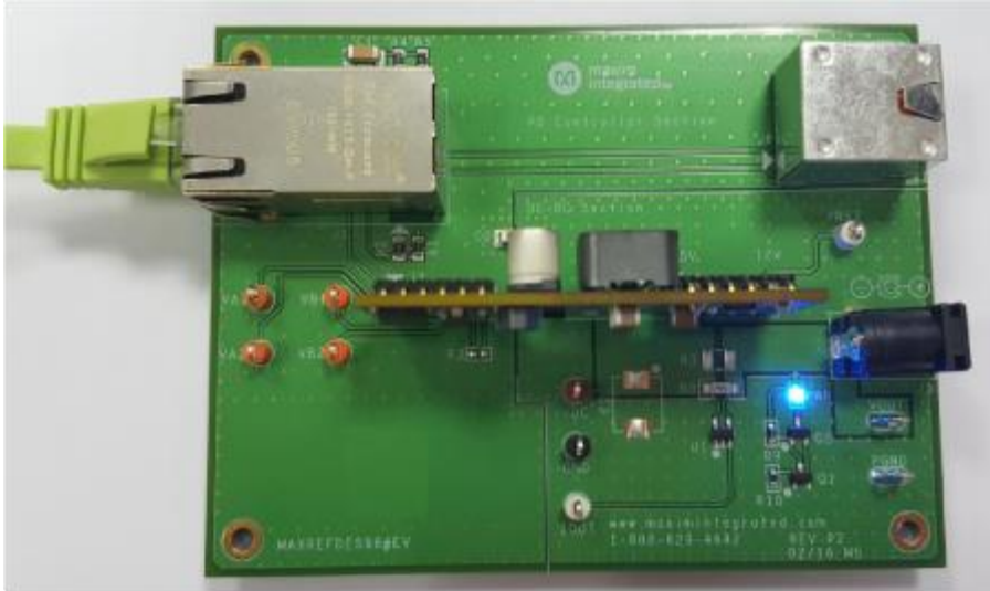
Figure 6. When the MAXREFDES108# board works, the PWR LED on the MAXREFDES98EV# board lights up.
