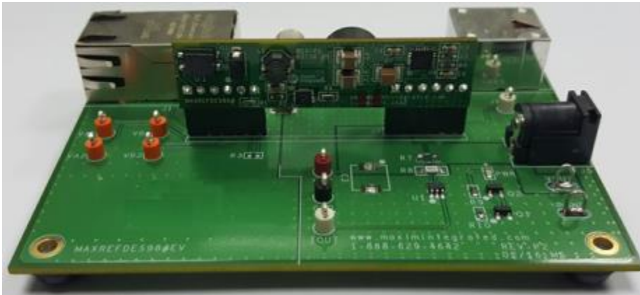
Figure 5. MAXREFDES98# connected to the MAXREFDES98EV#.
