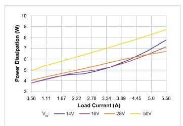
**Figure 6** — Power dissipation at 25°C case temperature,  $V_{OUT} = 26V$
