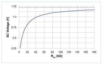
Figure 24 — Temporary margining to a lower value using optional resistor  $R_{SC}$
