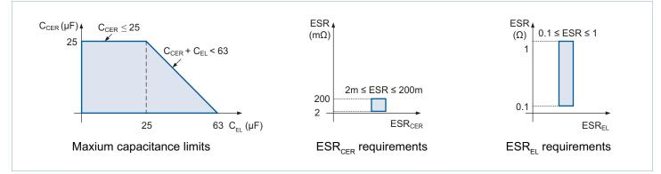
Figure 28 — Output capacitance limits
