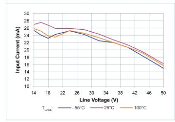
Figure 3 — Disabled input current vs. line voltage
