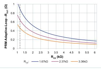
Figure 25 — Programming the adaptive-loop compensation with  $R_{VC} = 1k\Omega$
