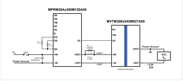
MPRM28Ax360M120A00 + MVTM36Bx045M027A00 isolated adaptive-loop configuration for negative supply
