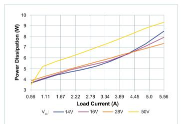
**Figure 18** — Power dissipation at  $-55^{\circ}$ C case temperature,  $V_{OUT} = 26V$
