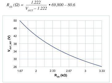
Figure 23 — PRM output voltage set point determined by value of R<sub>OS</sub>
