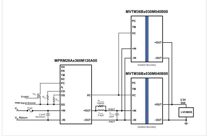
MPRM28Ax360M120A00 + two MVTM36Bx030M040B00s for isolated 180W-logic supply
