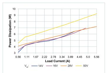
**Figure 12** — Power dissipation at 100°C case temperature,  $V_{OUT} = 26V$
