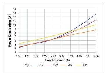
**Figure 8** — Power dissipation at 25°C case temperature,  $V_{OUT} = 36V$
