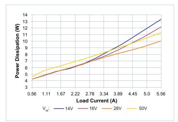
**Figure 20** — Power dissipation at  $-55^{\circ}$ C case temperature,  $V_{OUT} = 36V$
