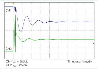
Figure 27 — Example CV to CC transition with fast load slew rate
