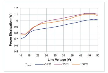
Figure 4 — No-load power dissipation vs. V<sub>IN</sub> at nominal trim
