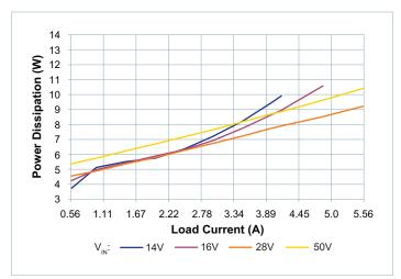
**Figure 14** — Power dissipation at 100°C case temperature,  $V_{OUT} = 36V$
