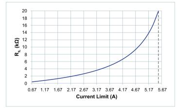
Figure 26 — Programming the constant-current limit threshold with  $R_{lL}$
