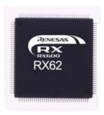
The **uEZGUI-RX621-35QT** includes a 100MHz Renesas RX621 or RX62N microcontroller running the open source uEZ® + FreeRTOS software platform. The RX62N has 512KB of internal Flash memory, 96KB of internal SRAM, a 10/100 Ethernet Media Access Controller (MAC), a USB full speed device/host/OTG controller, up to six UARTs, one CAN channels and a collection of serial communications interfaces. The unit also includes 512KB of external PSRAM.
