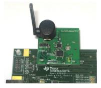
The CC2530-CC2591EM can be plugged into the SmartRF05EB. Please refer to the SmartRF05EB User Guide for more information about SmartRF05EB (http://www.ti.com/lit/pdf/swru210)
