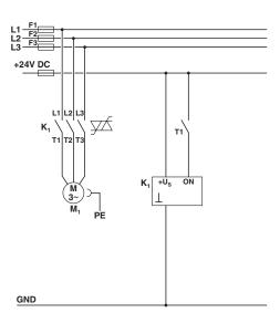
Structure with CONTACTRON Main and control current path for '2 in 1' hybrid motor starter K1 = '2 in 1' hybrid motor starter T1 = Right
