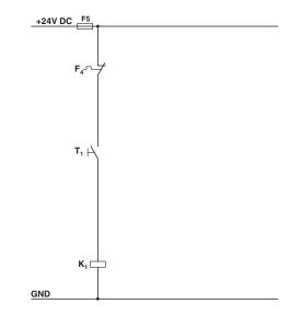
Conventional structure Control current path contactor K1 = Right contactor T1 = Right F4 = Motor protection relay
