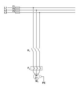
Conventional structure Main current path reversing contactor K1 = Right contactor F4 = Motor protection relay
