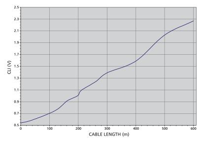
Figure 4-4: Cable Length Indicator Output
