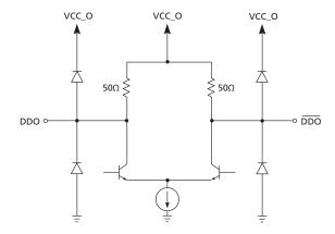
Figure 3-3: Output Circuit
