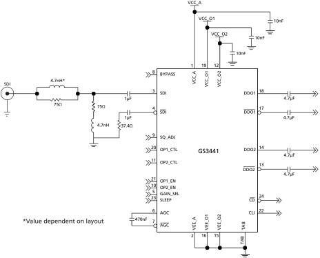
Figure 5-1: GS3441 Typical Application Circuit
