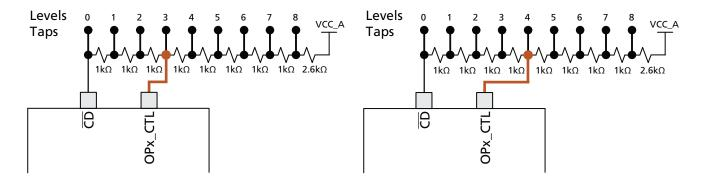
Figure 4-2: Resistor Divider Loopback Example #1 (Function Level 3 from Table 4-5)
