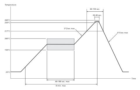
Figure 6-1: Maximum Pb-free Solder Reflow Profile
