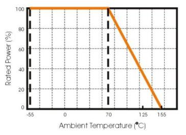
Fig 1 Maximum dissipation in percentage of rated power as a function of the ambient temperature for CR06, CR03, CR03, CR02
