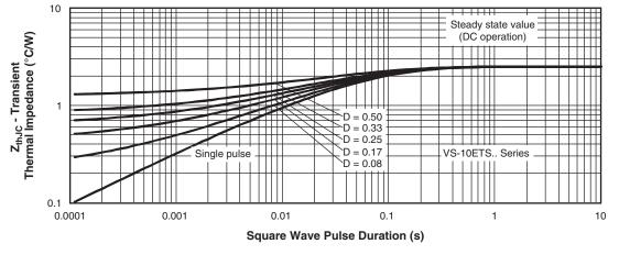
Fig. 8 - Thermal Impedance Z<sub>thJC</sub> Characteristics
