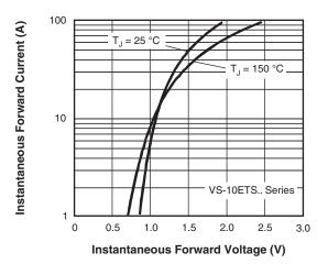
Fig. 7 - Forward Voltage Drop Characteristics
