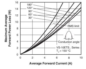
Fig. 3 - Forward Power Loss Characteristics
