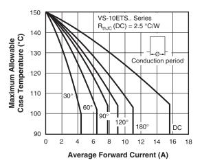
Fig. 2 - Current Rating Characteristics
