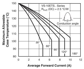
Fig. 1 - Current Rating Characteristics
