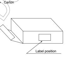
The aluminum package in which the reel is supplied also has the label attached to center of one side.
