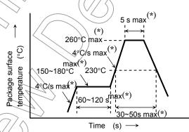
• The products are evaluated using above reflow soldering conditions. No additional test is performed exceed the condition (i.e. the condition more than (\*)MAX values) as a evaluation. Please perform reflow soldering under the above conditions.
