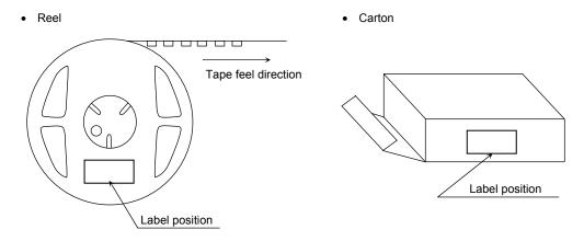
The aluminum package in which the reel is supplied also has the label attached to center of one side.
