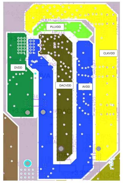
Figure 102. Fourth Layer of DAC3482 Layout Showing Power Layers. Layout Example from DAC3482EVM Rev H
