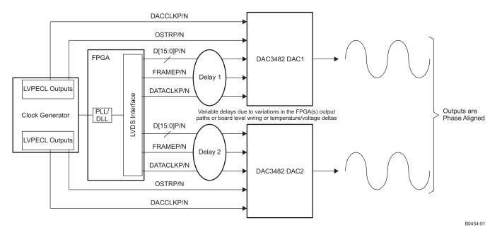
Figure 87. Synchronization System in Dual Sync Sources Mode with PLL Bypassed
