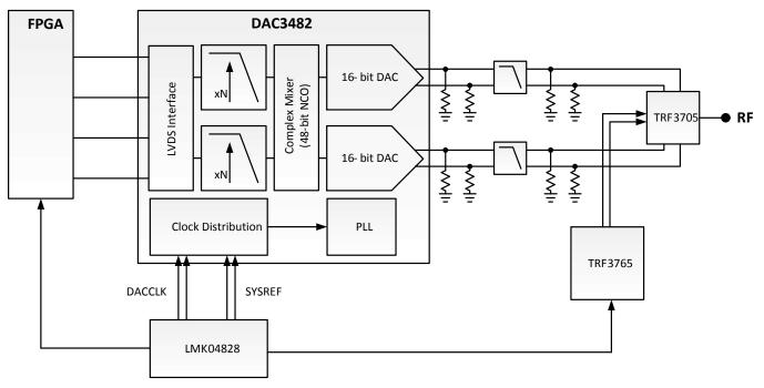
Figure 91. Dual Low-IF Wideband LTE Transmitter Diagram
