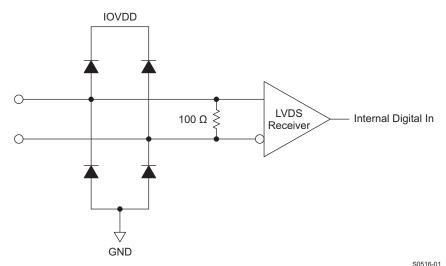
Figure 81. D[15:0]P/N, DATACLKP/N, FRAMEP/N, SYNCP/N and PARITYP/N LVDS Input Configuration
