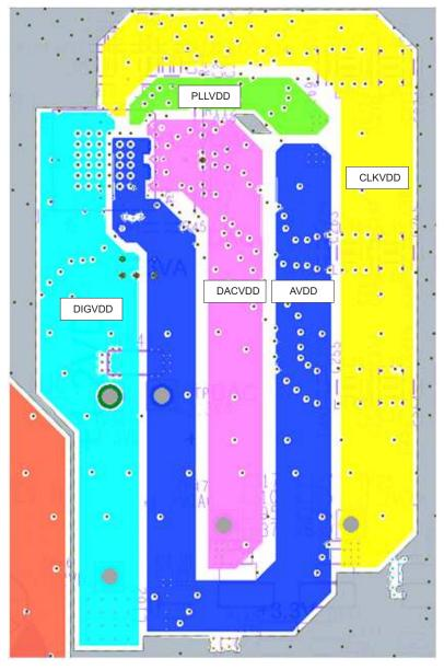
Figure 101. Third Layer of DAC3482 Layout Showing Power Layers. Layout Example from DAC3482EVM Rev H
