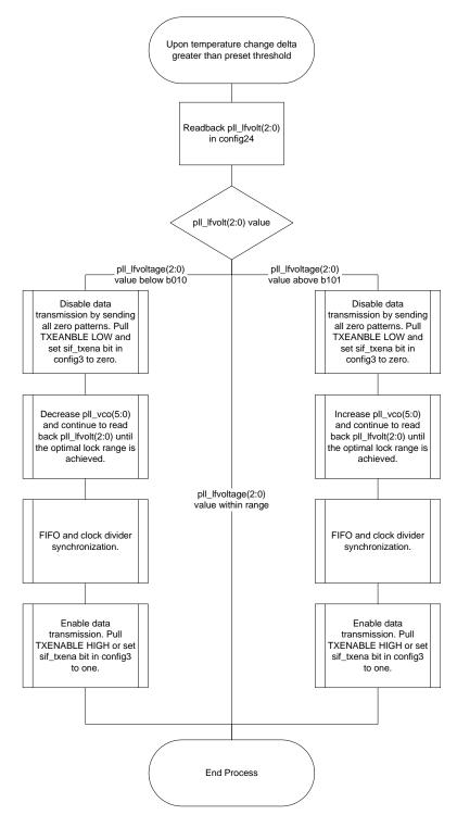
Figure 58. Example PLL Lock Status and Adjustment Algorithm
