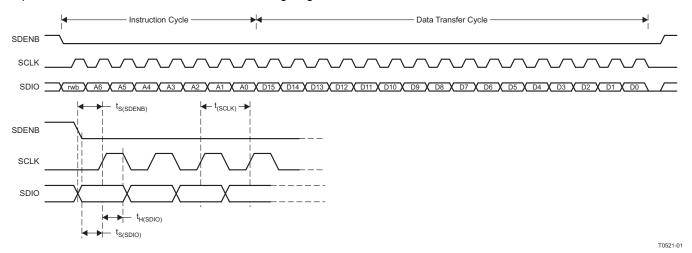
Figure 49. Serial Interface Write Timing Diagram
