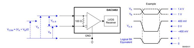
Figure 82. LVDS Data Input Levels
