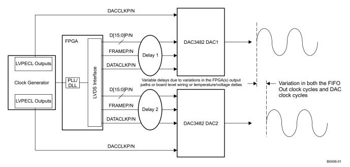
Figure 90. Multi-Device Operation in Single Sync Source Mode
