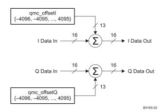
Figure 74. Digital Offset Block Diagram
