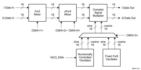
Figure 69. Path of Complex Signal Mixer
