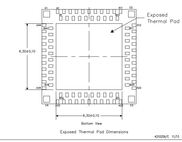
NOTE: All linear dimensions are in millimeters
