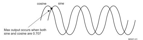
Figure 72. Maximum Output of the Complex Signal Multiplier
