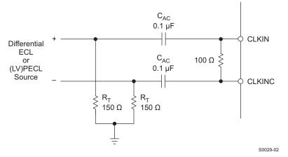
Actual RT value depends on differential clock driver output termination recommendation. It is driver type dependent.
