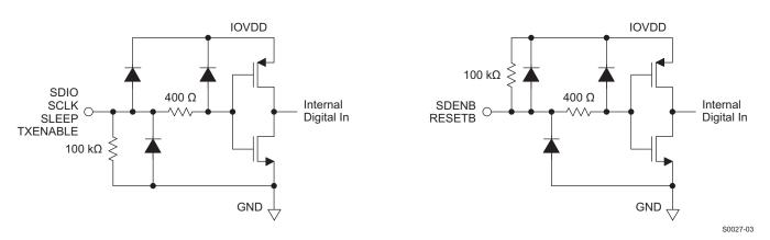
Figure 84. CMOS Digital Equivalent Input
