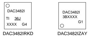
Figure 103. Date Code Location for RKD Package Option and ZAY Package Option
