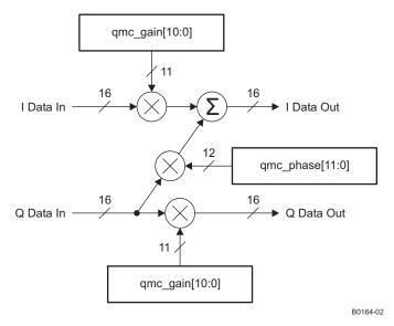
Figure 73. QMC Block Diagram
