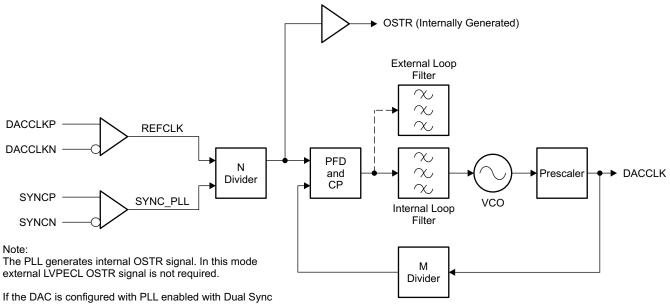
If the DAC is configured with PLL enabled with Dual Sync Sources mode, then the PFD frequency has to be the predefined OSTR frequency.
