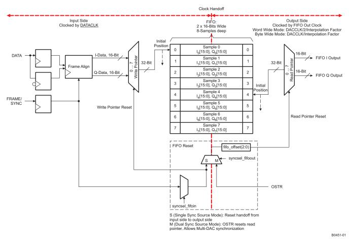
Figure 53. DAC3482 FIFO Block Diagram
