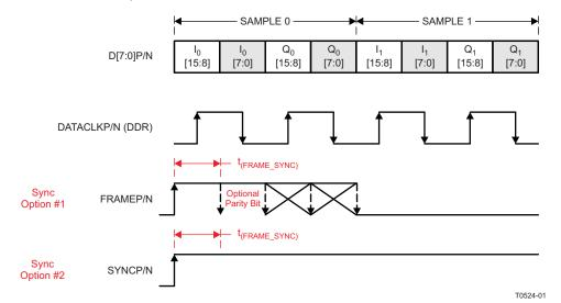
Figure 52. Byte-Wide Data Transmission Format
