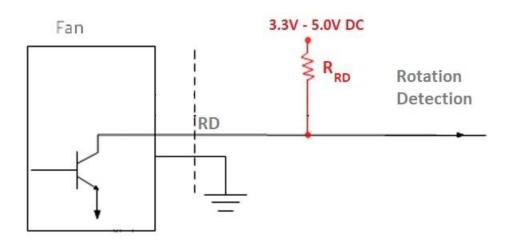
NB: Suggested pull-up resistor value of 1K to  $10 \text{K}\Omega$
