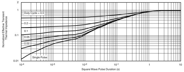
Normalized Thermal Transient Impedance, Junction-to-Foot
