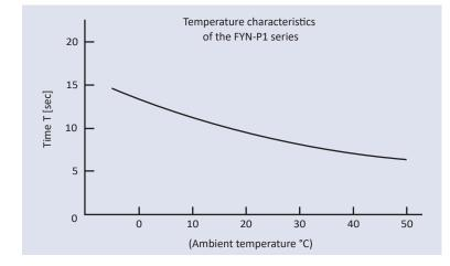
Damper characteristics vary according to the ambient temperature. In general, the damper characteristics become weaker as the temperature increases, and become stronger as the temperature decreases. This is because the viscosity of the oil inside the damper varies according to the temperature. When the temperature returns to normal, the damper characteristics will return to normal as well. The changes in the time it takes for the lid to close are shown in the graph to the left.
