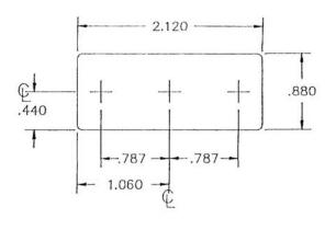
NOTE: A template can be made to these dimensions; or the 3 screw holes can be drilled (as per the instruction sheet) on these centers.
