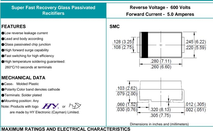
Rating at  $25^{\circ}$ C ambient temperature unless otherwise specified. Single phase, half wave ,60Hz, resistive or inductive load.
