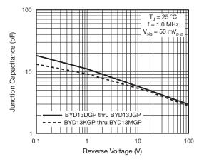
Fig. 6 - Typical Junction Capacitance
