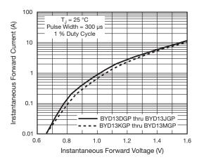
Fig. 3 - Typical Instantaneous Forward Characteristics
