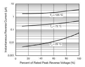
Fig. 4 - Typical Reverse Characteristics
