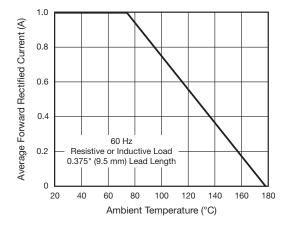
Fig. 1 - Forward Current Derating Curve
