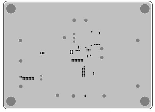
Figure 2. PCB Layout—Inner Side (2<sup>nd</sup> Layer)
