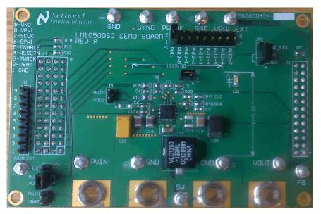
Figure 1. LM10500 Evaluation Board
