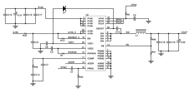
Figure 10. LM10500 Evaluation Board Schematic (Part I)
