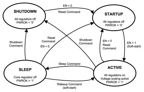
Figure 7. PWI Slave Operation States Diagram
