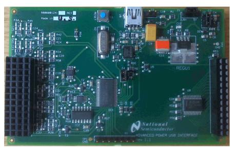
Figure 2. USB2PWI Interface Board
