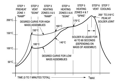
Figure 5. Typical Solder Heating Profile
