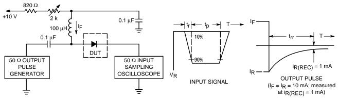
Notes: 1. A 2.0 k $\Omega$  variable resistor adjusted for a Forward Current (I<sub>F</sub>) of 10 mA. 2. Input pulse is adjusted so I<sub>R(peak)</sub> is equal to 10 mA. 3. t<sub>p</sub> » t<sub>rr</sub>
