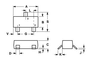
NOTES: 1. DIMENSIONING AND TOLERANCING PER ANSI Y14.5M, 1982. 2. CONTROLLING DIMENSION: INCH. 3. MAXIMUM LEAD THICKNESS INCLUDES LEAD FINISH THICKNESS. MINIMUM LEAD THICKNESS IS THE MINIMUM THICKNESS OF BASE MATERIAL
