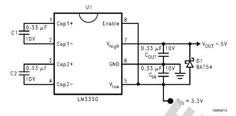
FIGURE 2. Step-Up Converter
