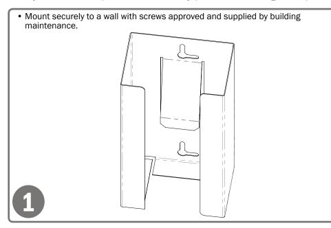
Dispenser can be mounted onto a BOWMAN<sup>®</sup> door or wall hanger through the cutout in the back.
