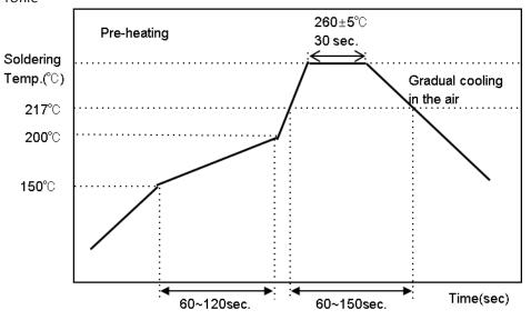
[Reflow Soldering Conditions]
