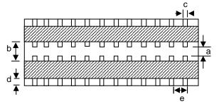
(Substrate for bending strength test)
