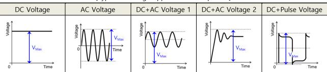
[Types of Voltage Applied to the Capacitor]
