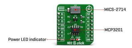
The resistance of the MiCS-2714 sensor does not change linearly with the gas concentration, so a proper calibration must be performed prior to using it for absolute gas concentration measurement applications. The impedance changes the most when used with low gas concentrations. As the atmosphere gets saturated with gas, the impedance changes slower.
