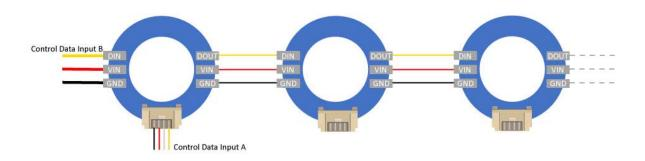
When multiple light rings are connected together, the control signal can be input from the Grove SIG pin or from the DIN input. However, Grove VCC has insufficient power supply and needs to input power from VIN.
