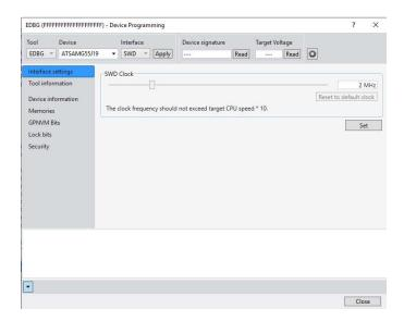
**Figure 3. Programming Clock Frequency**
