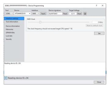
Figure 4. Device Signature and Target Voltage
